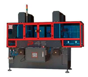
The P45 Carton Sealer by Spanish company Ear-Flap, is a multi format, carton sealing (taping) machine that is capable of taping cartons up to 500mm in width, 500mm in height and 700mm in length and achieve rates up to 15 cartons per minute. It can tape both the top and bottom of a carton and has automatic carton height and width adjustment settings.
