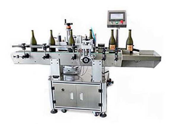
This machine is suitable for applying labels on cylindrical objects, such as xylitol, round cosmetics bottles, beer and liquor bottles, etc. Can apply labels by full circle or half circle, and front and back side of the whole circle.
