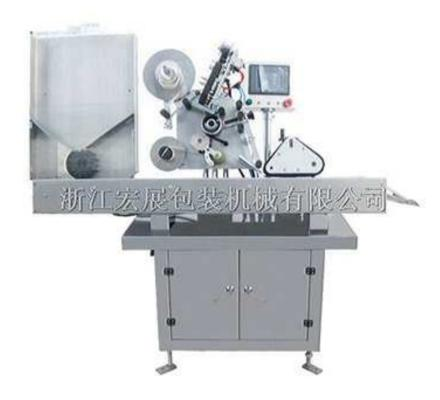
HTP series labeling machine is suitable for cylindrical or flat glass bottle and plastic bottle, stick lable on bottle circle, semi-circle as required position Two conveyor type: horizontal and vertical. Flat bottle can single side label or double side label.
