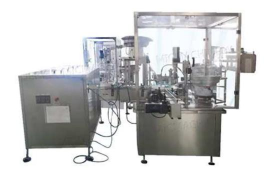
This e liquid filling plugging capping machine is suitable for: Essential oil, eye-drops, syrup, eliquid and other dose liquid.
