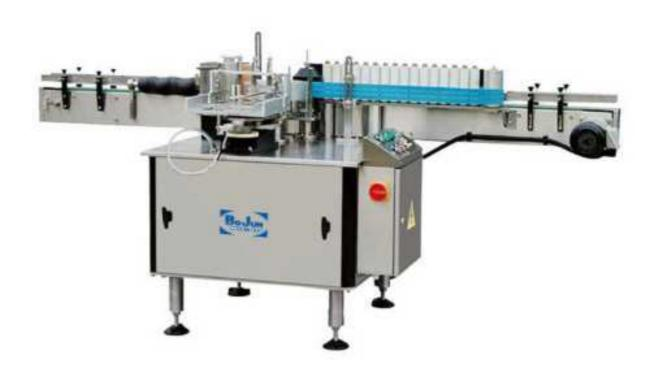
The machine suits for the consecutive paper label-sticking of cylinder vessel such as round glass, plastic and polyester bottle, it can automatically fetch label, smear clue and stick. Under the controlling of the dector.
