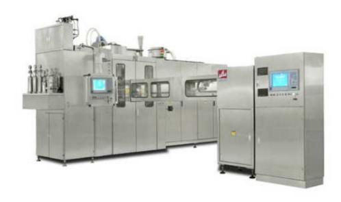
Apply sterilizing packing and suitable for the liquid filling product in pharmaceutical and chemical and food industry.
