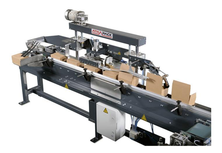
It automatically folds the wings and closes the box lid. When the flaps are folded, the lid is closed by the hot-glue bonding technique (it is made by spraying the glue to some required points with a gun). The format change is easily performed by the electronic system with easy settings.
