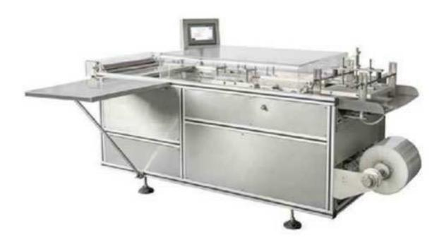
The semi-auto cellophane wrapping machine is a packaging machine manually that always overwrap the product with BOPP film. The semi-auto cellophane wrapping machine is wildly used in cosmetics, healthcare, perfume etc.
