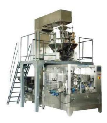
This packaging machine is suitable for high-precision metering bag filling and sealing of powder materials. Put some bags in the bag and pass the vacuum
