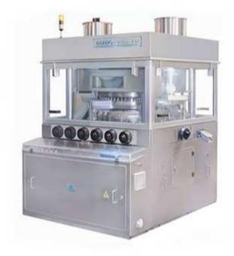
Prism TabXpress-IV is a High Speed Double Sided Rotary Tablet Compression Press suitable for millennium batch size production.
