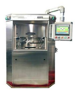
This machine is one kind of double side rotary tablet press machine, which can press granular materials into round shape tablet, irregular tablet or double-side engraved tablet. This machine is mainly used in pharmaceutical, chemistry, foodstuff, electronic industries.
