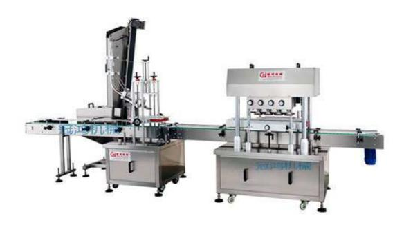
Linear Screw Capping Machine integrates automatic bottle feeding, automatic capping, automatic capping, automatic bottle discharging. The operation is stable and reliable, and the operation is simple and convenient. It is a standard plastic and metal thread circle for food, beverage, and medicine and health care products.
