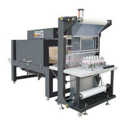
Working process: Cutting Wrapping Shrink Bottle Packing Machine USES shrink film to wrap in the product or package, after heating, shrink film to shrink the product or package, fully show the appearance of goods, improve the product display, and increase the sense of beauty and value. It is a kind of automatic and unmanned packaging machine, which can be used in automatic packaging line.
