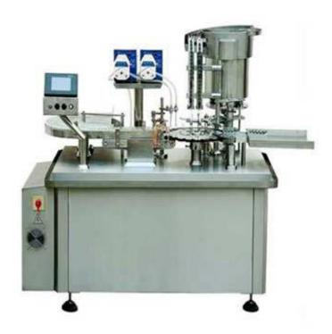
Vial filling and plugging machine for the application of round Vial bottle or similar ones, auto accomplish product filling, plug unscrambling, plug placing. The machine is composed by a load turntable, conveyor, and peristaltic pump &fill nozzles, plug sorter, Plug placer system. The bottle loading/unloading is done manually, through loading turntable Ø500mm, or able to directly from a production line. It is designed and made accordance to GMP regulation.
