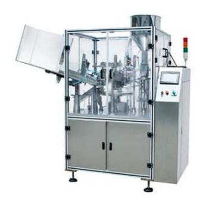
GZJ-100B Plastic (composite) hose and sealing machine is mainly used for a driving principle. Use segmentation mechanism driven turntable mounted fixture for intermittent operation, automatic filling and complete internal and external heating, sealing, play yards, trimming, finished withdraw a series of functions. Filling accurate measurement, the heating time is stable, adjustable, sealing beautiful appearance, neat, strong, health, trimming smooth.
