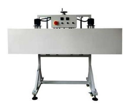
Electric shrink tunnel is used for shrinking sleeve labels of small bottles' body or sealing bottles' caps/necks.
