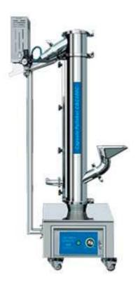
C&C100C series Capsule Polisher has achieved double functions of capsule polishing and elevating. Inlet of the machine can be connected with any model of capsule filling machine, and outlet with capsule sorter and metal detector, so that to realize the production line of capsule polishing, elevating, sorting and detecting.
