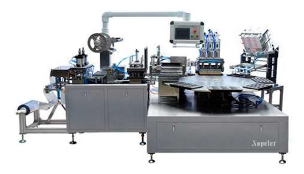
The equipment can Suitable for 12 sticks glue with 4\*3 pattern packaged, can automatically complete molding bubble shell, punching and cutting, bubble shell transition, automatic paper card, thermal bonding, finished product delivery and other functions.
