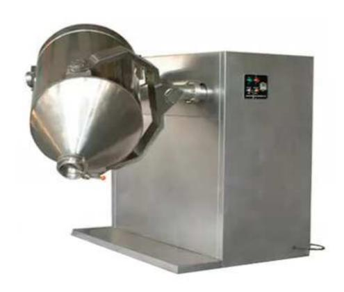
The barrel for charging the materials is driven by the driving shaft. The barrel body carries on the repeated level movement, rotation, turning and other complex movements so that the materials will carry out the three dimensions and complex movements along the barrel body so as to realize the various movements of the materials. Through disseminating, gathering, agglomerating and mixing to realize uniform mixing.
