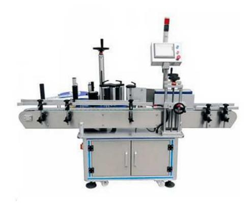
The fully automatic vertical round bottle labeling machine, can achieve automatic positioning labeling, single standard, double standard, label distance interval adjustment. This machine is suitable for PET bottles, metal bottles, glass bottles etc. It is widely used in food, beverage, cosmetic pharmaceutical industries.
