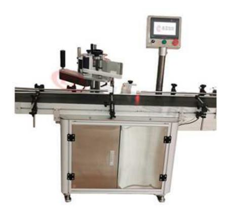
It is suitable for labeling or self-adhesive film on the side of various items, such as switching power supply, paper box, fan, carton, etc. It is widely used for side labeling of large products, and labeling of side surface objects with a wide range of specifications.
