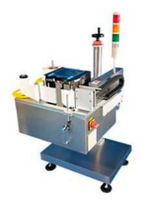
Suitable for different size carton diagonal corner labeling, widely used in pharmaceutical, cosmetic, logistics and other industries - Carton Corner Sealing Labeling Machine.
