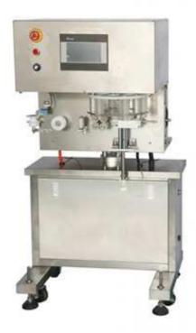
CI-200 Cotton Inserter is economical and easy to operate. The machine can automatically cut off the belted cotton and insert it into the container accurately and speedy. This fully automatic cottoner inserts a predetermined length of cotton, rayon or polyester coil into containers at speeds up to 45 cpm.
