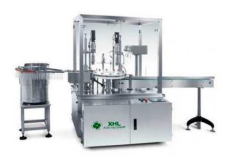
The series of products are mainly used for aseptic filling of serum, cell culture medium, etc. in such industries as medicine, biology, etc. The whole production process is completed under the protection of 100-level laminar flow and aseptic isolation, ensuring aseptic production and conforming to the new version GMP requirements. The production line inherits internationally
