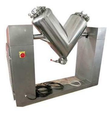
V shape blender is an asymmetric machine of high efficiency. It is generally applicable in chemical, food, pharmaceutical, fodder, ceramic or metallurgical industries to mix powdery or granular materials. It features reasonable and simple structure, operation in closed environment, convenient feeding and discharging, manual or vacuum material feeding. Its container is made of stainless steel and can be cleaned easily. Many enterprises adopt it as the basic equipment for granulation.
