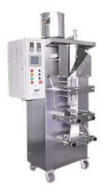
DXDY-320 liquid automatic packaging machine process parts are all made of stainless steel. With high-level balance tank or self-priming pump quantitative filling, straight heat sealing and cutting, bag size, packaging weight, sealing temperature adjustment convenient and reliable, the machine can production date ribbon print, edge Seal, back seal, photoelectric tracking.
