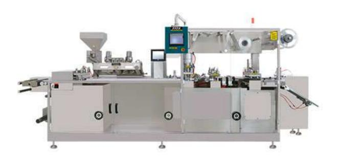
The machine has the reasonable design, novel structure. Equipped with automatic feeding system, packing testing, plate cooling integral, waste recycling and other devices, can automatically complete the package material feed, blister molding, drug filling, packing testing, heat sealing, batch number, indentation, blanking, scrap plate rejection, finished product output and other process. The production process is intuitive, easy operation and maintenance, complete functions.
