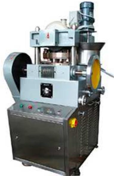
This machine is used to press the granular raw material into the round tablets or various geometric shaped tablets, it is especially caters for small scale production. When pressing the tablets, the rotary disc speed and filling depth of material can be adjustable.
