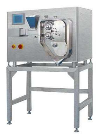
MRCH120 roller compactor is newly self-developed equipment for lab use and pilot test on basis of foreign advanced technology. It features compact structure, simple operation, easy cleaning and maintenance and effective to test the parameter for the future batch production. It can be widely utilized for pharmaceutical, food and chemical industry.
