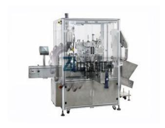
The filling sealing and capping machine is suitable for medication, food and chemical industry. It got the functions of filling with heat preservation, sealing film, capping and locking automatically with the materials of high viscosity paste. This bottle filling and capping machine equips with PLC controller and human interface, makes the structure compact, operation easy and performance stable.
