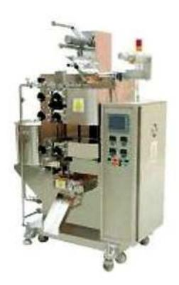
This machine is a three-section roller vertical packaging machine designed to achieve automatic packaging of liquid materials sealing three sides or four sides. It is suitable for the packaging pesticides, daily use chemical, food, medicine and other liquid materials.
