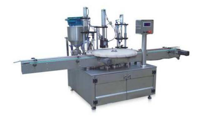
The cream filling machine adopt piston filling method, it suitable for the skin care and cosmetic cream, such as the vanishing cream, foundation cream. The Turntable help to fixed the short and round containers when material filling.
