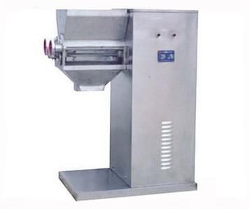
YK granulator machine is a kind of small swing granulator. It is used to make moist or dried powder substance into the needed granular particles. Chuan Chu Company mainly supplies YK60, YK90 AND YK160A oscillating granulators. They are typically used in laboratories and also extensively applied in pharmacy, chemical industry, food, pottery and plastics, etc.
