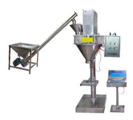
As a machine manufacturer, we are committed to producing machines of higher quality. Semi automatic auger powder filling machine is a new machine launched by the company in combination with the latest technology. Auger type powder filling machine is suitable for weighing and filling various powder and mixed powder like materials, such as additives, fertilizers, flour, coffee powder, milk powder, washing powder, monosodium glutamate, solid drinks, sugar, seasoning and other powder products.
