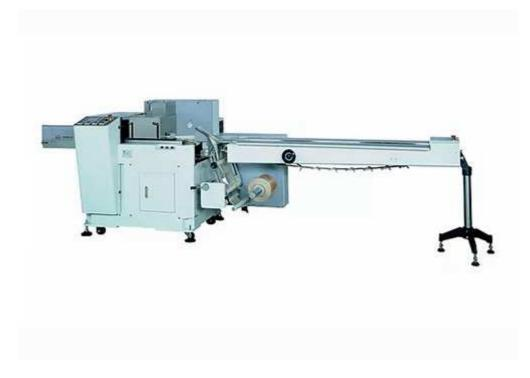
Inverted packing machine model. Packing film roll fed from the base of the machine. Delicate products are then transferred directed on to the film with the long seal then been made above the product.
