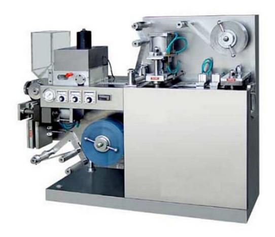
Flat Plate Automatic Blister Packaging Machine is specially developed for dosage room in hospital, mini-pharmaceutical factory, mini-motor test workshop, and medicine institute. Pressed to mold, this machine is flat plate structure and convenient to operate. The dimension is small and the stroke length is adjustable. It suits for aluminum plastic package for any shape of objects, such as capsule, tablet, pellet, sugarcoated tablet, leisure candy, milk tablet, mini metal etc.
