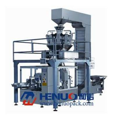
This automatic line, by combining rotary packer, multi-head weigher, elevator and support platform, is suitable for packing all kinds of granules such as candy, nuts, dried fruits, currant, fudge, peanut, seeds, pip, chocolate, crackers, coffee beans, rice
