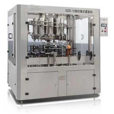
This filling machine is an automatic filling and capping machine. It adopt piston filling type, it could be applicable for all kinds of oil, fruit &vegetable sauce (with or without solid piece), granule drink quantify filling and capping, no bottles no filling and capping, PLC control system, easy operation.
