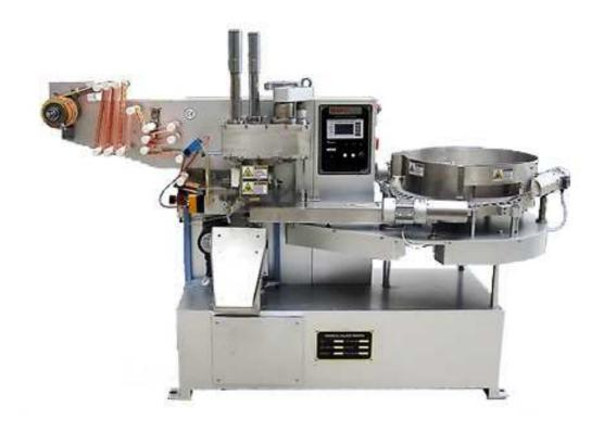
SWP150 Lollipop Packaging Machine is applicable to wrapping lollipop into single twist style. Frequency converter for speed adjustment, PLC control system is used on the machine; Parameter setting and paper cutting adjustment is achieved by operator-machine interface. It is of the function of automatic running and compensating, twisting and healing of paper as well as parameter display during running.
