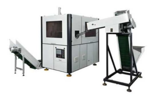
ES series, two-step method fully automatic blow molding machine is the most stable machine in our company. The maximum capacity is 1.5L, suitable for blowing with PET as raw materials of any shape carbonated beverage bottles, mineral water bottles, cosmetics bottles and packaging container.
