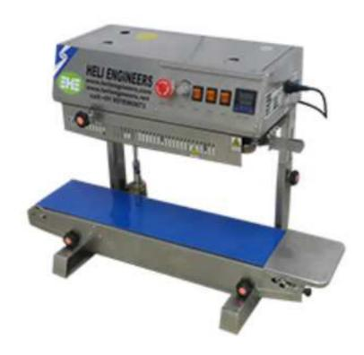
The continuous bag sealing machine is semi automatic solution for closing / sealing filled bags / sachets / pouches using continuous band sealing heaters. Available in vertical and horizontal models to meet various bag sealing / closing requirements.
