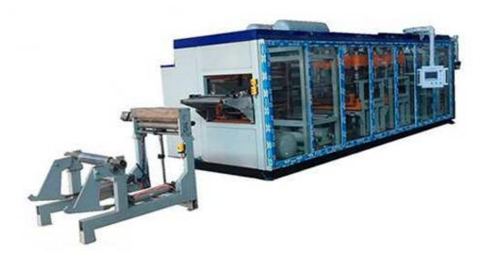
IM-HP model is a trim-in-place type thermoforming machine with rules steel knife for automatically In-line hole-punching for tray and container and clamshell.
