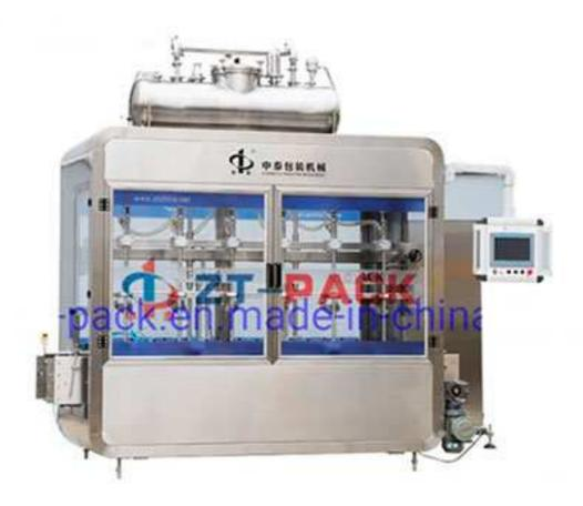
This fully automatic net weigh filling machine is ideal for filling liquid products such as cooking and edible oils into drums or large containers. It can automatically implement complete operations including container in-feeding, weigh filling, container out-feeding. This net weigh filler is widely used in foodstuff, pharmacy, cosmetic and chemical industries.
