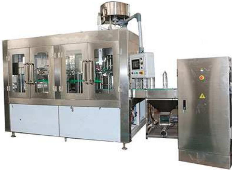
The carbonated beverage filling machine could be separated into 3 modules. The height of the bottle-out conveyor is adjustable. Bottles are conveyed to rinse, filler and capper through starwheel and conveyed out finally through the bottle-out conveyor. equipped with an alarm device for bottle block, bottle absence, cap absence and overload, the pet bottle soda filling machine meets the national food hygienic standard with high automation and easy to operate.
