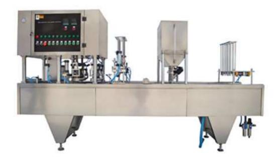
This machine is designed to fill and seal plastic cups or similar containers with liquid, cream and others. Whole process is fully automatic, including cup loading, cup filling, sealing, coding, and output. Cup filling machine series have capacities from 1500 to 16000 bph, satisfy most needs of factories. Top brands of components ensures a stable performance
