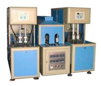
Semi Automatic Pet Blowing Machine adopts the new type double bend arm and four pull rodclamping structure. Cross direction; middle mound board is move parallel; the distance between two mold board is adjusted by the chain wheel.
