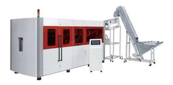
Full electric PET stretch blow molding machine is composed of three modules: prefrom elevator, perform unscrambler and host machine. It is equipped with automatic perform loading and unloading system. The machine is applicable for all shapes of drinking water bottles, carbonated bottles and juice bottles.
