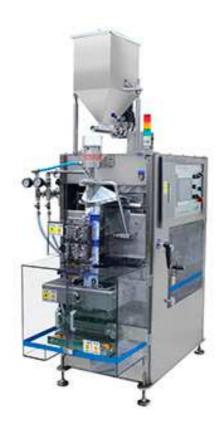
Vertical type automatic packaging machine and manufactured according to K.G.M.P standards. Inserting, sealing, cutting and position adjustment of product is possible. Almost no film loss.
