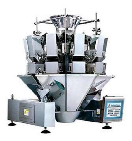
The 10-head high-precision multi-head weigher adopts a vibrator, which can automatically adjust the amount of vibration according to different target weight values, so that the feeding is more uniform and the combination is higher. The quantitative multi-head combination weigher is mainly used in conjunction with the automatic packaging machine, and is suitable for measuring and packaging granular and powder materials.
