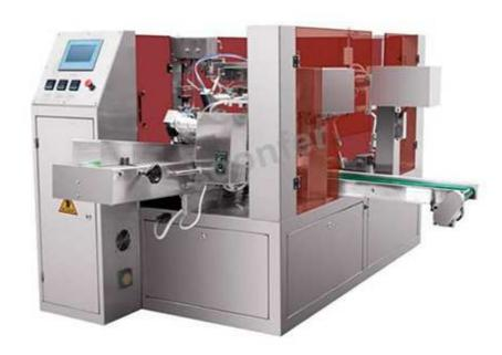
Automatic doypack juice liquid packing machine, Multi-functional packaging machine, can be used for packaging liquid, powder, and particle and shisha tobacco.
